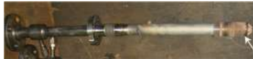
Pilot nozzle of DLN combustor
